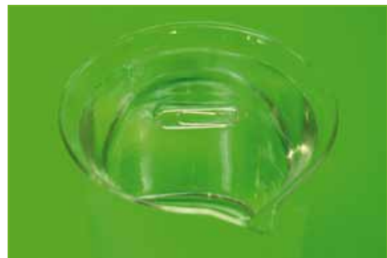
Surface tension of water (cohesion)
